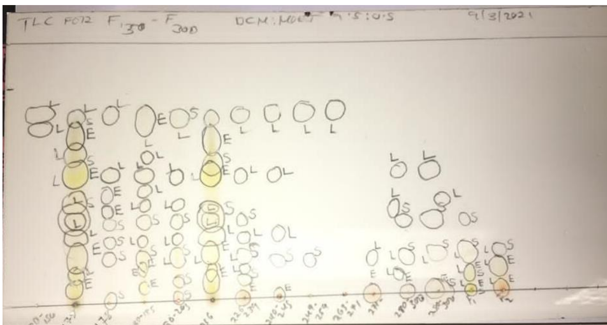
Figure 4: Figure (d): Isolated fractions as visualized under the naked eye, short wavelength & long wavelength
