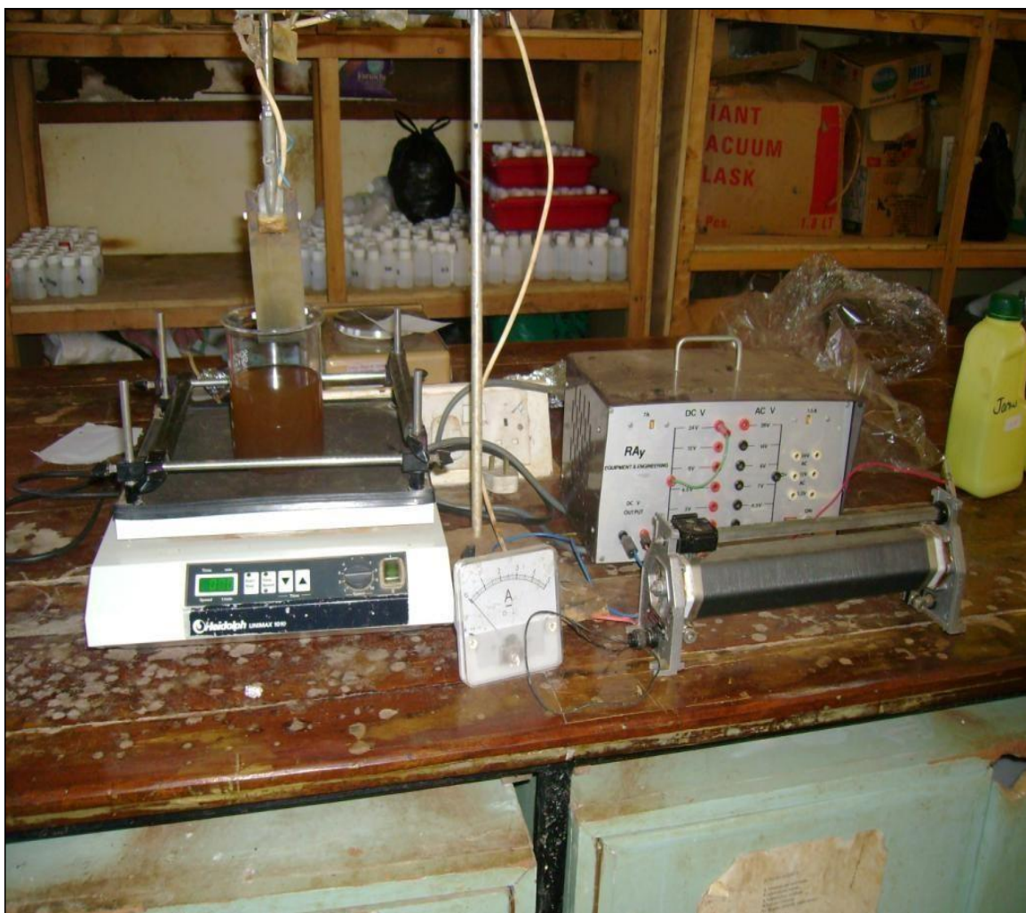
Scheme 3. 1: Electrochemical cell set up for Azo dye degradation, a photo taken from Pwani University Chemistry laboratory
