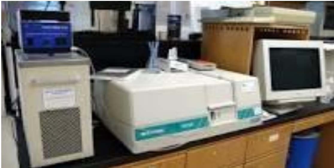
Scheme 2. 9: (a): A photo of Ultraviolet-Visible Spectrophotometer taken from Pwani University Biological lab
